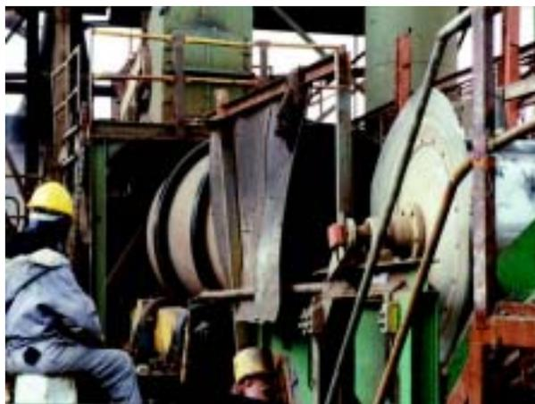
Photo 9: Operation Qeto: Centrifugal and electromagnetic machine that separates ferrous and non-ferrous or non-metallic scrap. Photo credit: South African Department of Defence.
