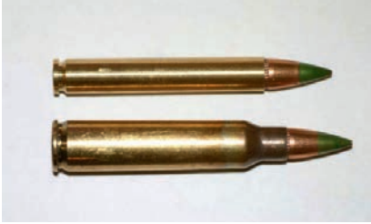
Photo 4 A comparison of the Knox Engineering Company 5.56 mm alternative cartridge geometry (top) and a standard 5.56 × 45 mm M855 cartridge (bottom)
