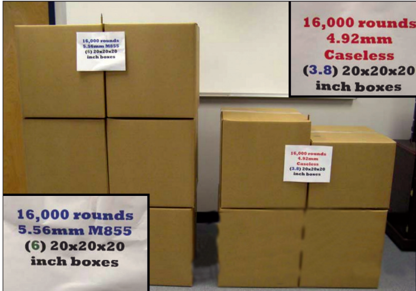
Photo 13 The volume of 4.73 × 33 mm high-ignition-temperature propellant caseless ammunition 53 (right) is about 37 per cent smaller than that of brass-cased US M855 5.56 × 45 mm ammunition (left)
