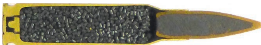
Photo 1 A sectioned (cutaway) 7.62 × 51 mm cartridge, showing the projectile, propellant, primer, and cartridge case
