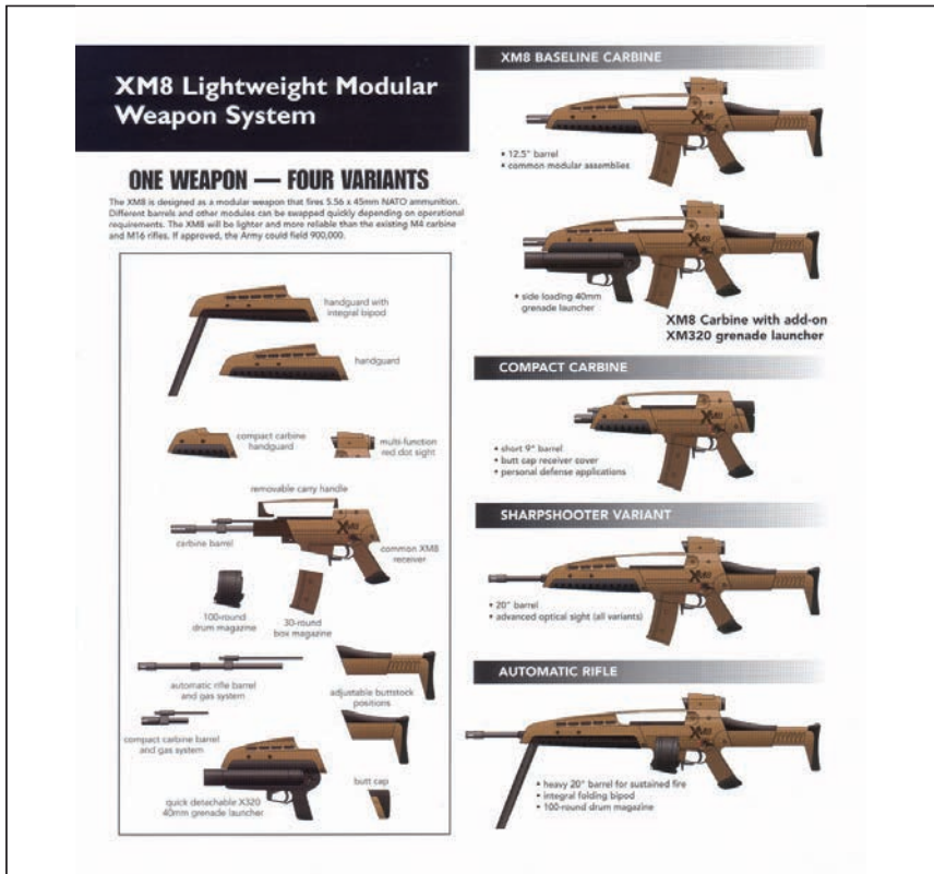
Photo 12 Heckler & Koch XM8 family of modular weapons. Note common receiver at centre right
