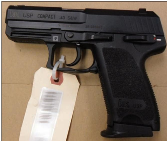
Modern firearms are increasingly built using a combination of materials such as plastic and metal. A single firearm can thus be marked with different methods, depending on the specific material of the component that is marked. These handguns carry a combination of stamped, laser-engraved, and cast marks.
