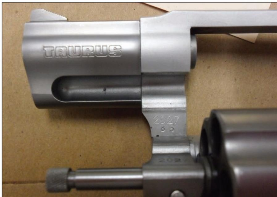
The typical features of dot peen marking are visible on this revolver. The numbers '2027' are created with a sequence of microdots, which yields a less defined and more discontinuous edge compared to the name 'TAURUS' on the barrel or the stamped '85' on the frame.
