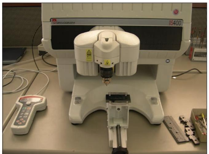
This scribing machine applies marks by mechanically engraving the surface. The quality of the mark is high, though the process is slower than other marking methods. Photo courtesy of GravoTech GmbH, Switzerland
