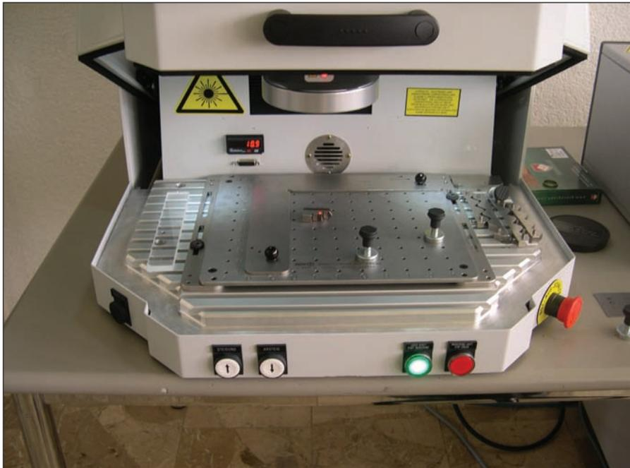
Since laser marking machines such as this one apply marks without any physical contact, the firearm does not need to be locked to avoid movement during the marking process. Once the object to be marked is positioned, the safety cabinet needs to be closed before the marking begins. Photo courtesy of GravoTech GmbH, Switzerland
