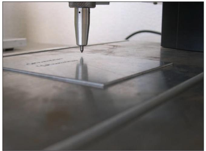
The carbide stylus oscillates, or vibrates, up to 300 times per second, resulting in up to five characters per second on flat, concave, or convex surfaces. Photo courtesy of GravoTech GmbH, Switzerland
