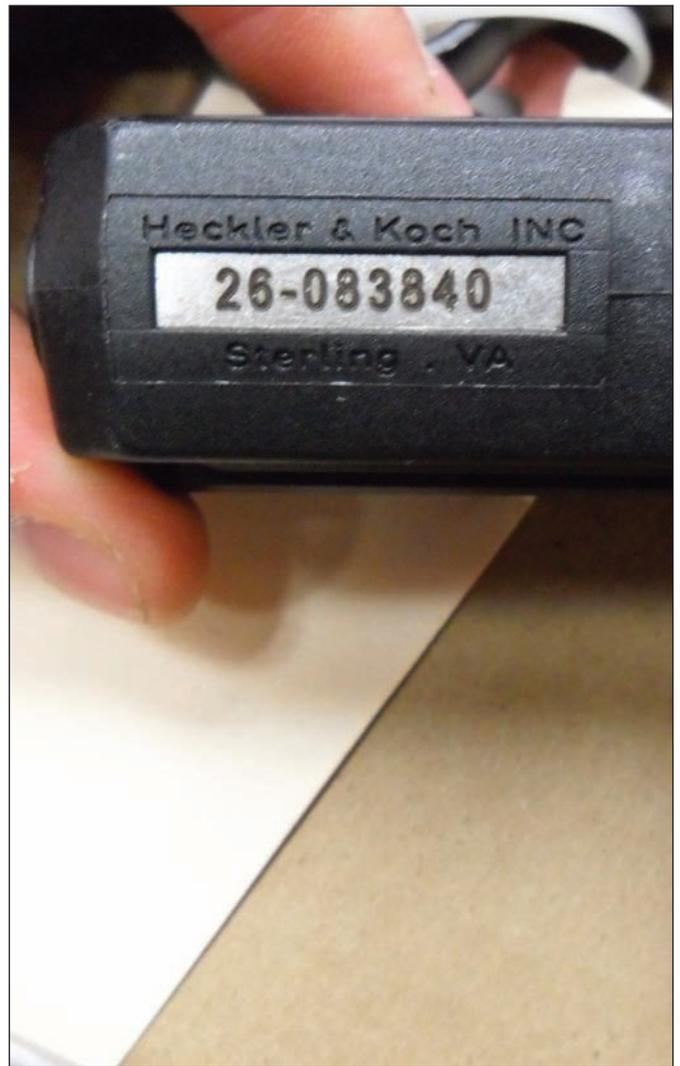
This handgun's receiver (or frame) has a metal tag bearing a stamped serial number.
