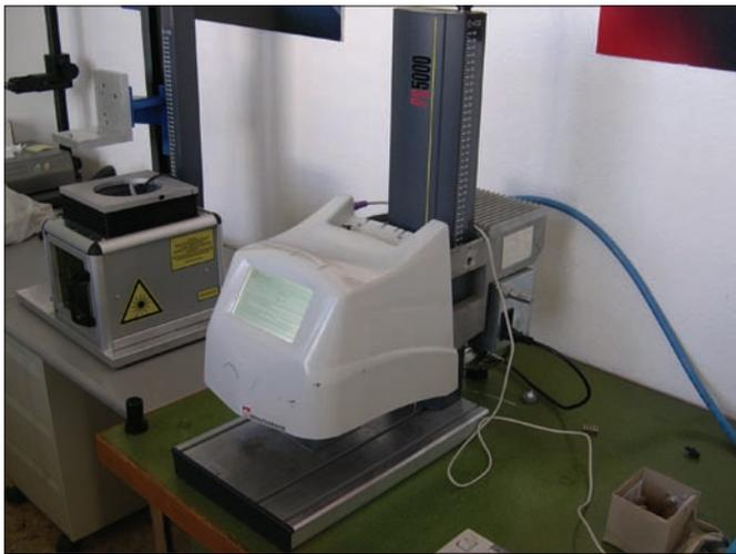
In this pneumatic dot peen marking machine, the air is supplied through the blue pipe. The user interface includes a built-in liquid crystal display (LCD) and an external keyboard (standard computer keyboard). Photo courtesy of GravoTech GmbH, Switzerland
