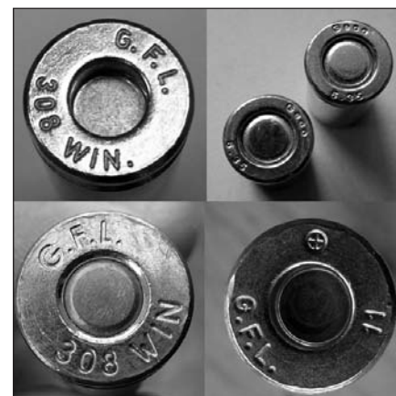
Figure 4 Examples of case marking
