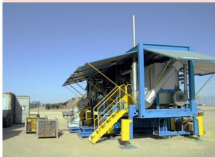
EODSolutions' Transportable Ammunition Destruction System (TRADS).
