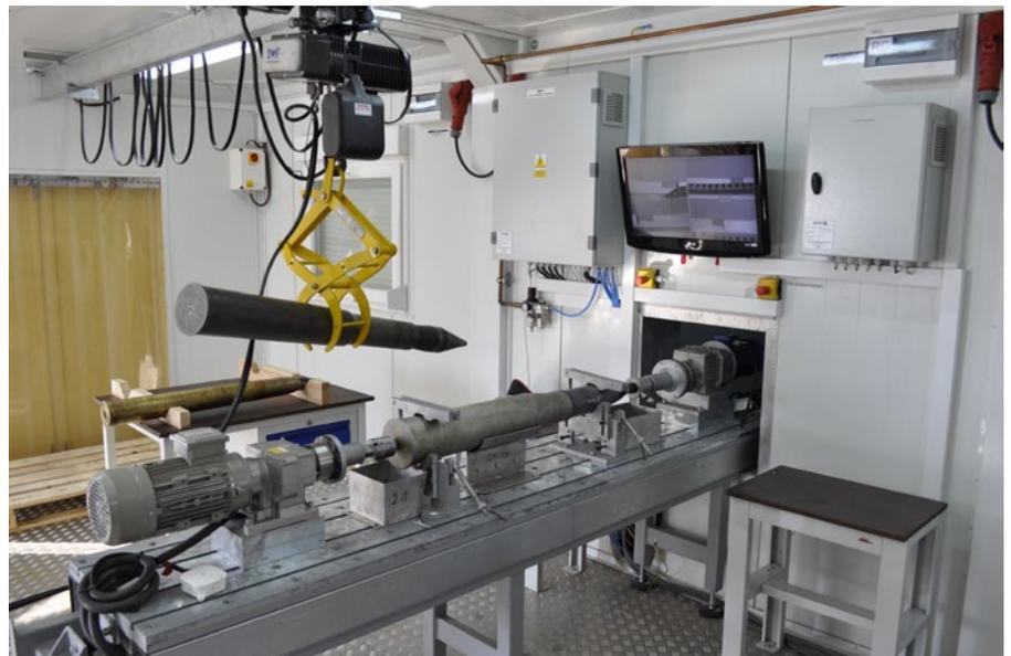
The ammunition disassembly component of JAKUSZ's Planetarium transportable system, processing a 100 mm UBK8 projectile. © JAKUSZ SZB/2011
