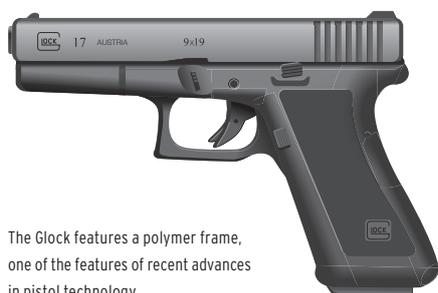
The Glock features a polymer frame, one of the features of recent advances in pistol technology.
