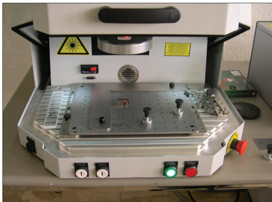
Since laser-marking machines such as this one apply marks without any physical contact, the firearm does not need to be locked to avoid movement during the marking process. Once the object to be marked is positioned, the safety cabinet needs to be closed before the marking begins.
