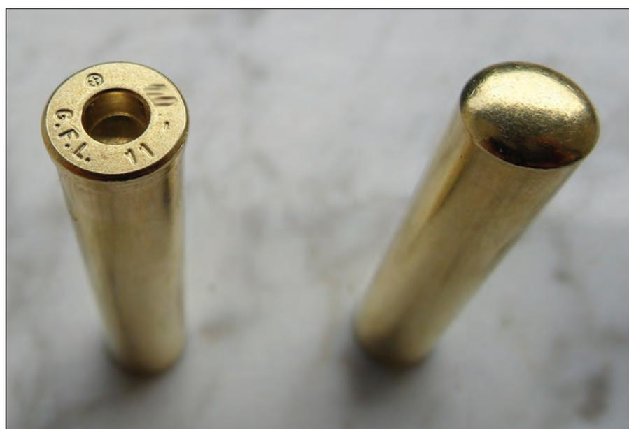
The case enters the machine as it appears on the right of the photo and exits with the marks and the lodging for the primer, as on the left. Photo courtesy of Fiocchi Munizioni. © Giacomo Persi Paoli
