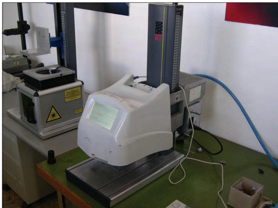
In this pneumatic dot peen-marking machine the air is supplied through the blue pipe. The user interface includes a built-in liquid crystal display and an external keyboard (i.e. a standard computer keyboard).
