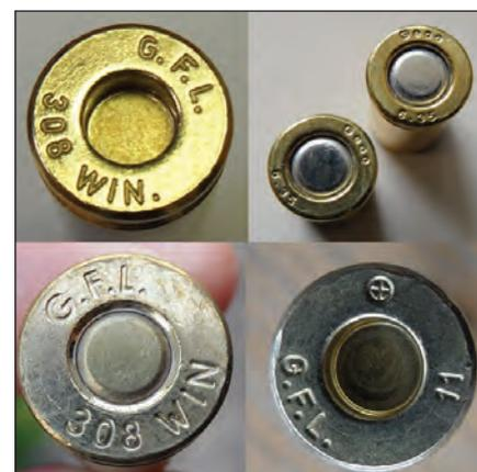
Left: a case for a .308 Winchester cartridge with (above) and without (below) the primer.
