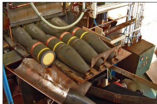
Photo (right): The saw-cutting of high-explosive projectiles to expose their energetic content, after which the components travel on a conveyor belt to the next station to melt out the explosives, Lübben, Germany, 2012. © Sprewerk Lübben GmbH
