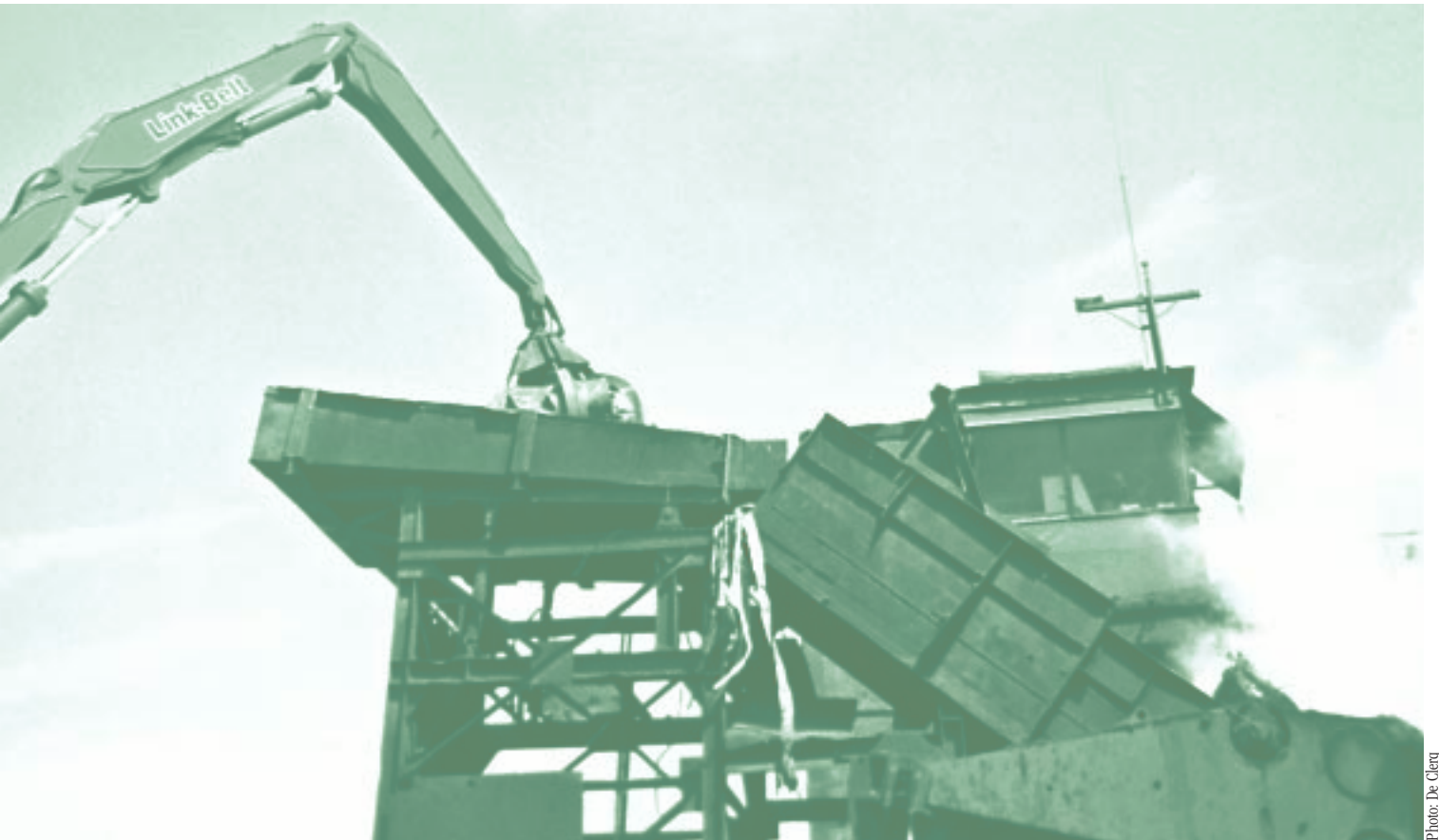
▲ Figure 4: Crane placing old vehicle containing firearms into giant shredder
