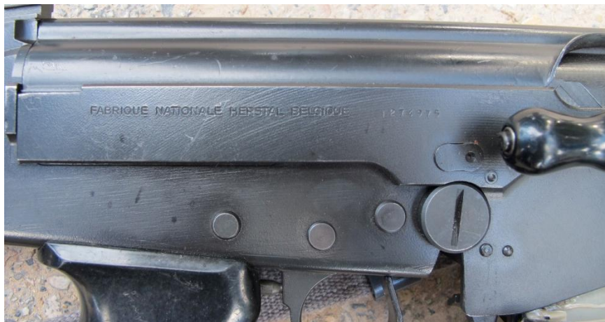
Picture 3 Serial number on the right-hand side of the upper receiver of a FN FAL rifle
