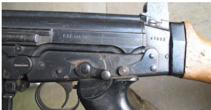
Picture 4 Serial numbers on left-hand side of the upper and lower receivers of a FN FAL rifle*
