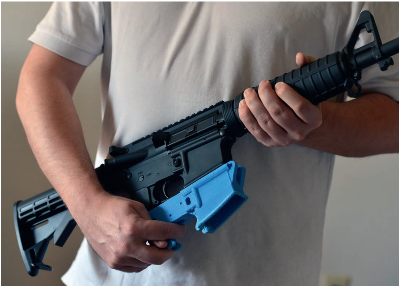
A man holds an AR-15 rifle and a lower receiver made of ABS plastic (in blue) that he made at his own home using a 3D printer, Maryland, United States, February 2012. Source: Jahi Chikwendiu/AFP Photo
