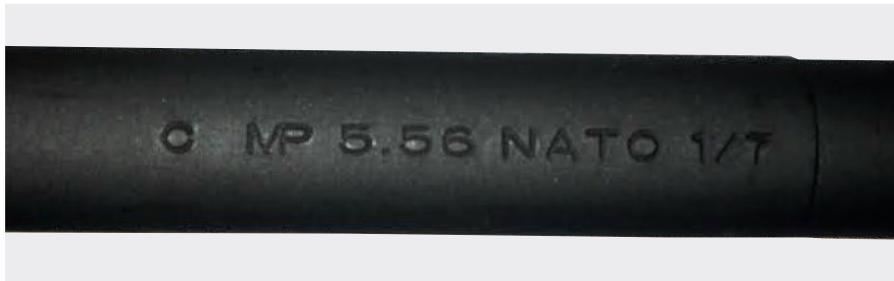
Note: The 'C' indicates the barrel was produced by Colt, 'MP' shows the barrel underwent a magnetic particle inspection, '5.56 NATO' indicates the barrel calibre, and '1/7' indicates the twist rate of the barrel's rifling.
