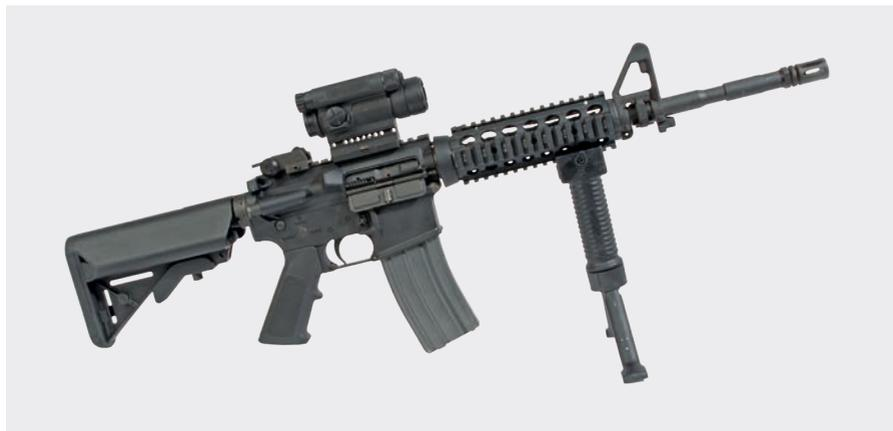
Note: The fore-end features accessory rails (in this case MIL-STD-1913 'Picatinny' rail) at the 12, 3, 6, and 9 o'clock positions, as well as a length of accessory rail on the upper receiver surface. An optical sight is mounted to the receiver accessory rail and a combined forward-grip/bipod is mounted to the 9 o'clock position of the fore-end 'quad-rail'.
