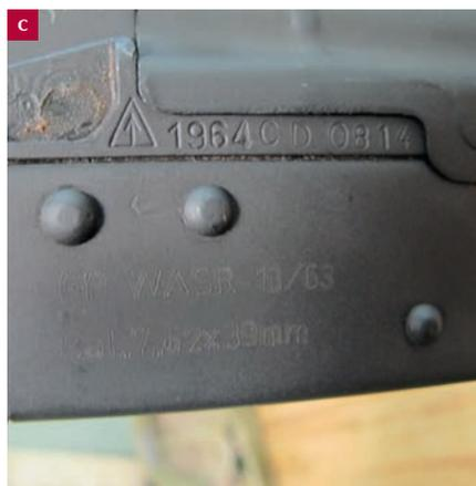
Note: (a) Markings ('Tabuk' and 'Cal. 7.62×39mm') on the right side of the rear sight block of an Iraqi Tabuk self-loading rifle. (b) Markings ('CQ' and 'CAL. 5.56MM') on a Chinese CQ self-loading rifle. (c) Markings ('WASR 10/63' and 'Cal. 7.62×39mm') on a Romanian GP WASR 10/63 semi-automatic rifle, rebuilt to Pistol Mitralieră md. 1963 standard. These are post-production markings engraved by an importer.
