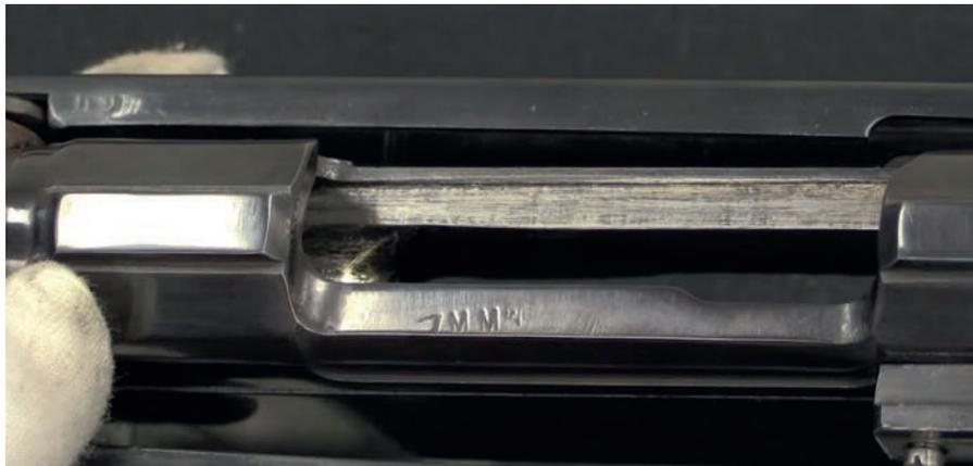
Note: The marking reads simply '7 M M'. After a chamber cast and test-fitting of a dummy cartridge, it was determined to be chambered for 7 mm Mauser (7 × 57 mm).
