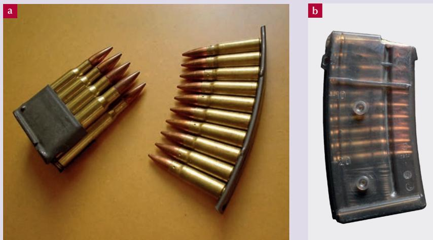
Note: (a) Examples of en bloc (left) and charger/stripper clips (right). (b) A (transparent polymer) removable box magazine for comparison.
