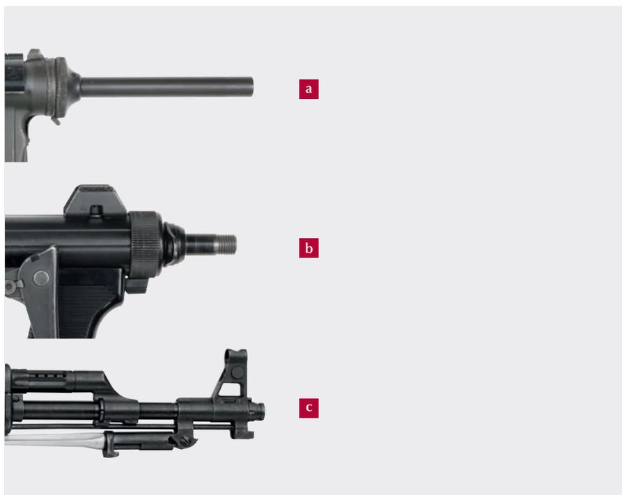
Note: (a) A bare muzzle on a US Guide Lamp M3 SMG; (b) A threaded muzzle on an Italian Beretta Model 125 SMG; (c) A thread protector or 'muzzle nut' on a Chinese Type 56-1 self-loading rifle (note also the under-folding integral bayonet).
