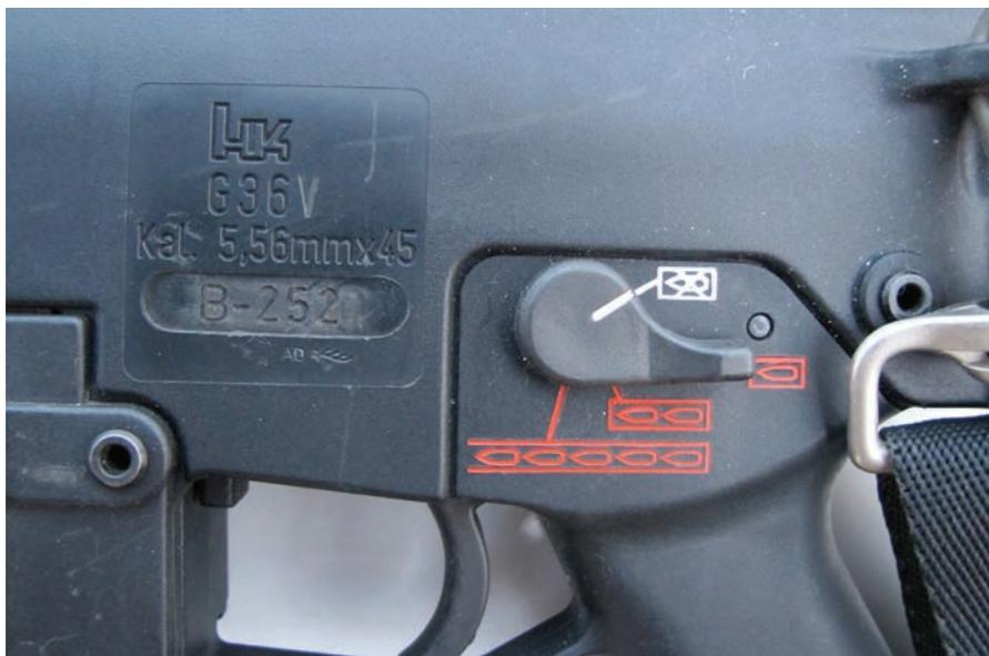
Note: The original serial number has been abraded and a new marking engraved.
