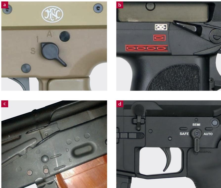
Note: (a) Markings (S, 1, A) on a Belgian FN Herstal SCAR-L self-loading rifle. (b) Pictographic markings on a German Heckler & Koch MP7 SMG. (c) Markings (D, E) on an East German MPI-KM self-loading rifle. (d) Markings (SAFE, SEMI, AUTO) on a British LANTAC LA-M4 self-loading rifle.
