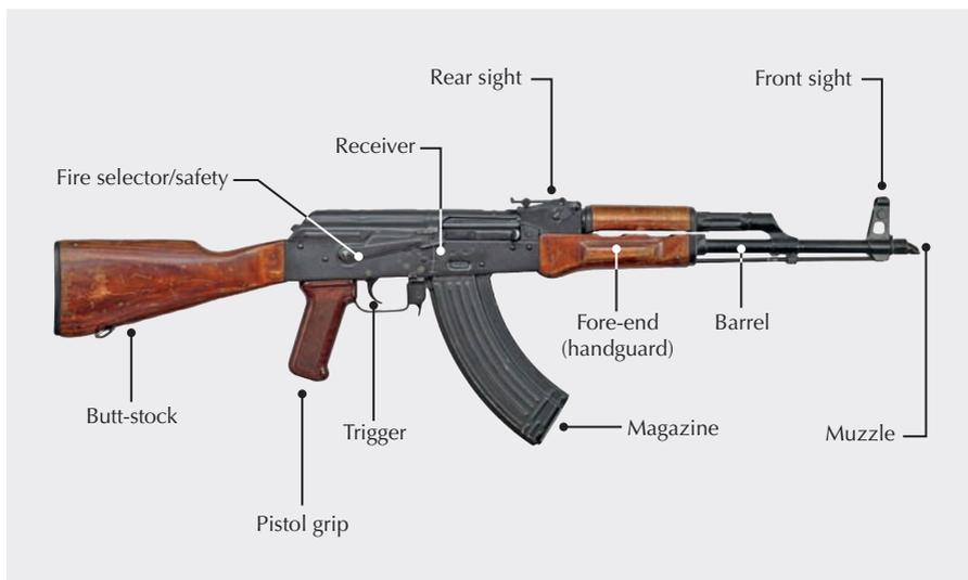
Note: With handguns, what might be termed the 'receiver' is typically referred to as a 'frame'. The slide of a self-loading pistol is similar to the 'upper' receiver of a rifle. Pistols by definition lack a butt-stock (ARES, 2017).
