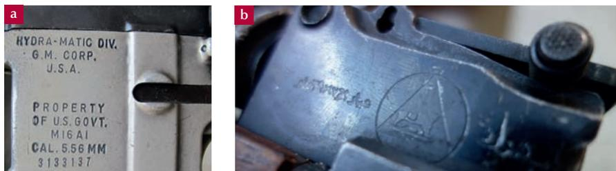
Note: (a) Government property markings on American Hydra-Matic M16A1. Note also the make/manufacturer, country of origin, calibre, and serial number markings. (b) Arsenal mark on an Iraqi Tabuk self-loading rifle.
