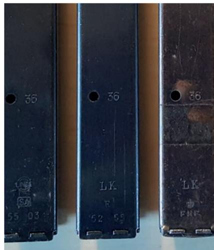
Note: These magazines show different construction techniques, metal finishes, and fonts used for the marking '36'.
