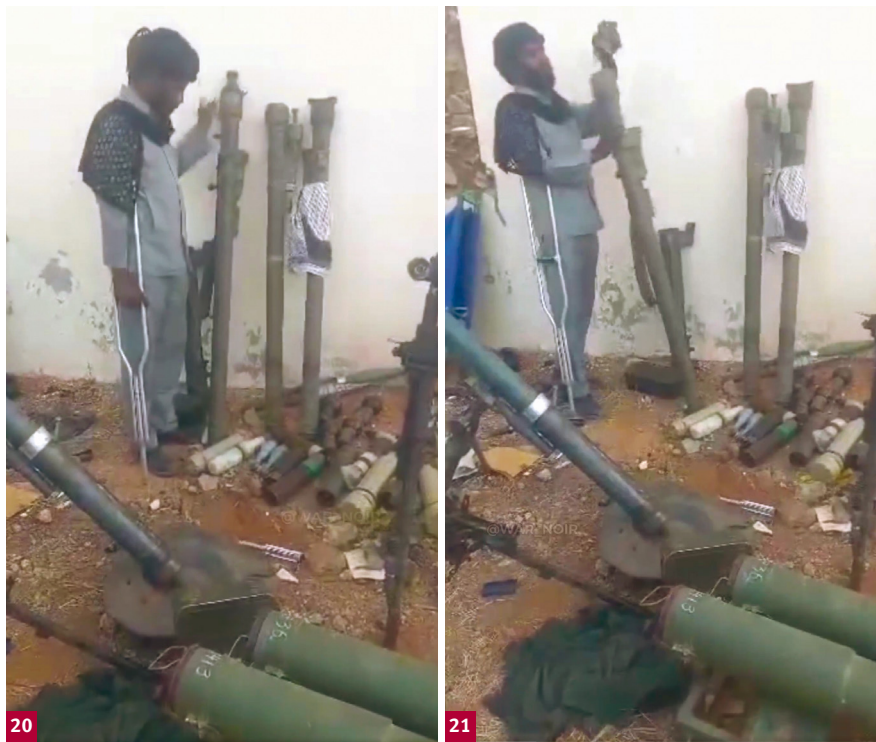
Notes: Imagery from a video of launch tubes for an Igla-1- and two Strela-2-pattern MANPADS (20–21) reportedly seized from the SAF by the RSF in late 2025. The video shows a man removing the cap from the Igla-1 tube, revealing the tri-cone nose of the missile. No gripstocks for Igla-1 MANPADS are visible in the video.
