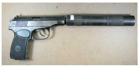
A 6P42 tear gas pistol, based on a Makarov PM, illegally converted to fire 9 x 18 'lethal' ammunition and fitted with a silencer. © Maxim Popenker, 2014
