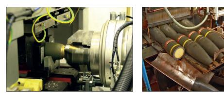
Photo (left): A projectile's nose fuse being removed remotely during the automated disassembly process, Kirikkale, Turkey, September 2007. © NATO Support Agency Photo (right): The saw-cutting of high-explosive projectiles to expose their energetic content, after which the components travel on a conveyor belt to the next station to melt out the explosives, Lübben, Germany, 2012. © Spreewerk Lübben GmbH
