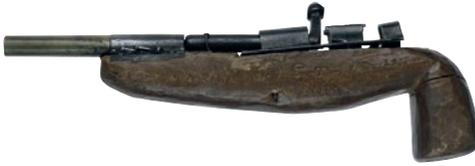
Note: This zip gun-type weapon originally used several strands of material taken from bicycle inner tubing to provide impetus to the firing pin.
